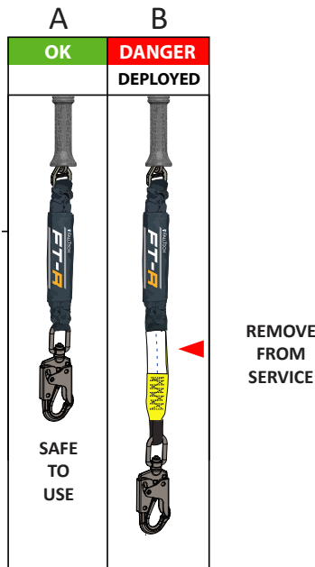
Figure 15 - Inspecting SRL-R Load-Indicating Energy Absorber
