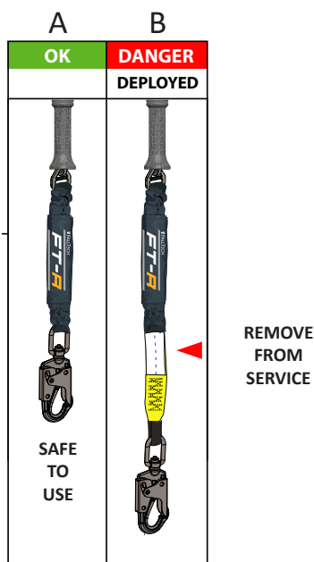
Figure 15 - Inspecting SRL-R Load-Indicating Energy Absorber
