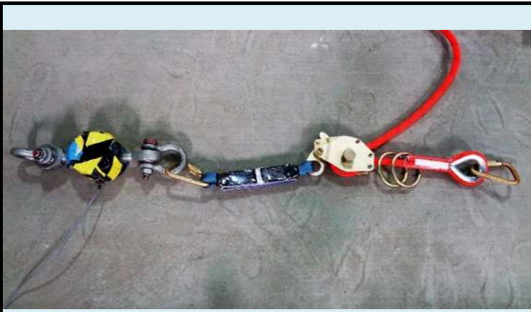
Figure 3: Kernmantle HLL Test Configuration Mockup
