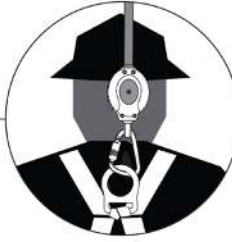
Figure 2A: 9' Max Web SRD Orientation and Acceptable Anchorage Range 9' Single-leg Attached to Dorsal D-ring Shaded area indicates Range of Allowable Connection from: Directly Overhead to as low as 5' Below User's Dorsal D-ring
