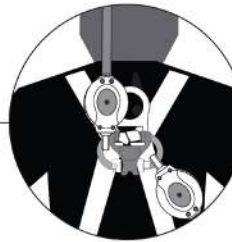
Figure 2C: 9' Max SRD Orientation and Acceptable Anchorage Range 9' Twin-leg SRD Attached to Full Body Harness Shaded area indicates Range of Allowable Connection from: Directly Overhead to as low as 5' Below User's Dorsal D-ring
