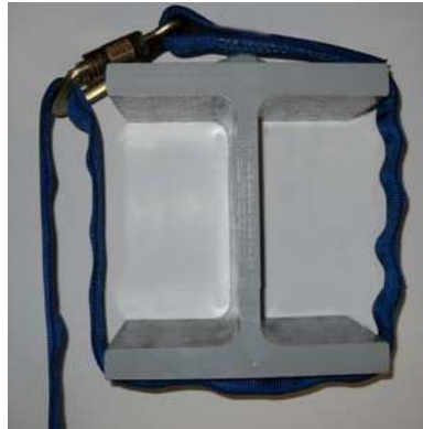
Incorrect Tie-Back Connection
