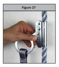
Step 5: The 8368 Fall Arrester is a trailing type. If a fall event occurs, the Fall Arrester will lock onto the VLL and arrest the fall.
