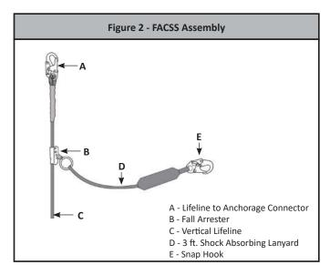
For the purposes of this manual, the system may be referred to as the equipment, Fall Arrester (Rope Grab), Fall Arrester Connector Subsystem (FACSS), the unit or the device. See Table 1 in Appendix A for ANSI/OSHA compliance information.
