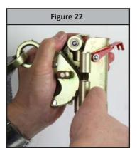
Step 5: Place the VLL in the rope channel, see Figure 23. Close the hinge and push in and down on the Locking Bolt Actuator with your thumb. Push the Locking Bolt Actuator down to lower the actuator pin. Allow the locking bolt to engage the lock receiver. Lower the safety latch, see Figure 24.
