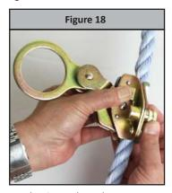
**Step 7:** Pull down on the ring and cam lever to ensure the Fall Arrester locks onto the VLL. These Fall Arresters are the trailing type. If a fall event occurs, the Fall Arrester will lock onto the VLL and arrest the fall.
