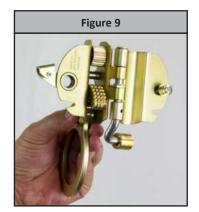
Step 4: Lift the ring to retract the cam assembly. See Figure 10. Place the VLL in the rope channel. See Figure 11.
