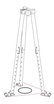
The FallTech 7275 Tripod is intended to provide a portable anchorage mount for the mounting of lifeline components of a comprehensive confined space entry, retrieval and rescue system. It should be erected above the opening of the confined space. It will accommodate round openings up to 5 feet in diameter and up to 4 feet square openings.
