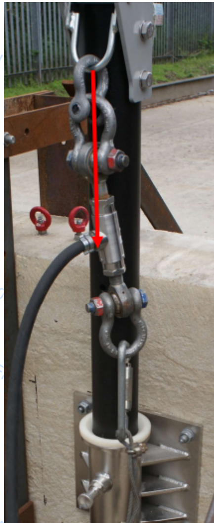
Figure 2 – Anchorage connector described as “DAC-WL” showing direction of test
