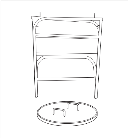
1. Position the guardrail over manhole lid while still covered.
