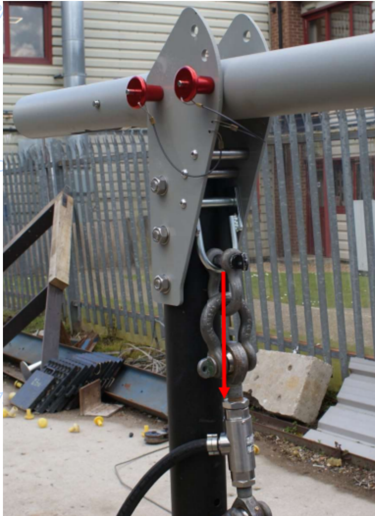
Figure 2 – Anchorage connector described as “DAC-HB” showing direction of test
