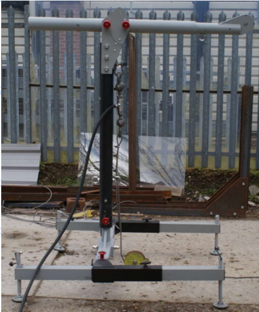
Figure 1 – Anchorage connector described as “DAC-HB”
