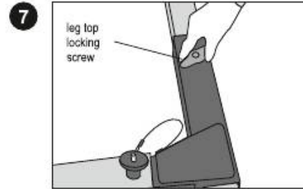
STEP 7- Tighten the leg top locking pin with provided screw locking to minimize the play between sections.
