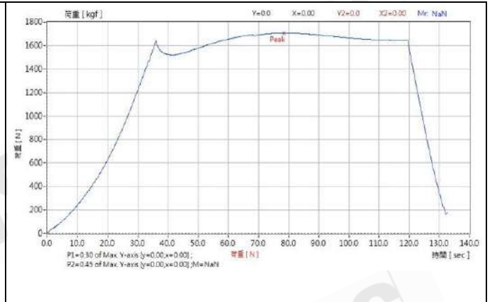
Photo "B" Static Strength – Sample No.1
