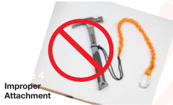
Figure 6 Tethering to FBH
