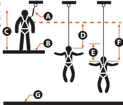
If there is a risk of a fall or if the only anchorage point is below the attachment points on the harness, it is essential to use a lanyard provided with an energy absorber. Before using a shock absorbing lanyard, ensure that there is sufficient fall clearance below the user to prevent any collision with the structure or ground.
