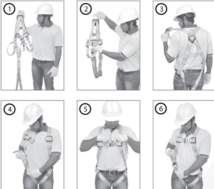
**Step 1:** Hold harness by grasping back D-ring. Shake harness to allow all straps to fall into place.
