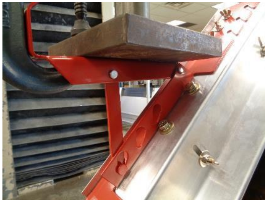
Photo No. 4 Adapter Plate Test - Roof Bracket (with Clamp) - Post Test Condition
