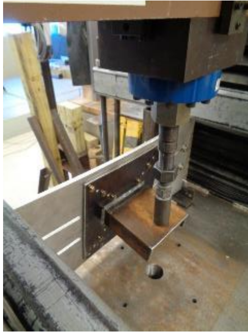
Photo No. 5 Spanner Plate Loading Test Set-Up
