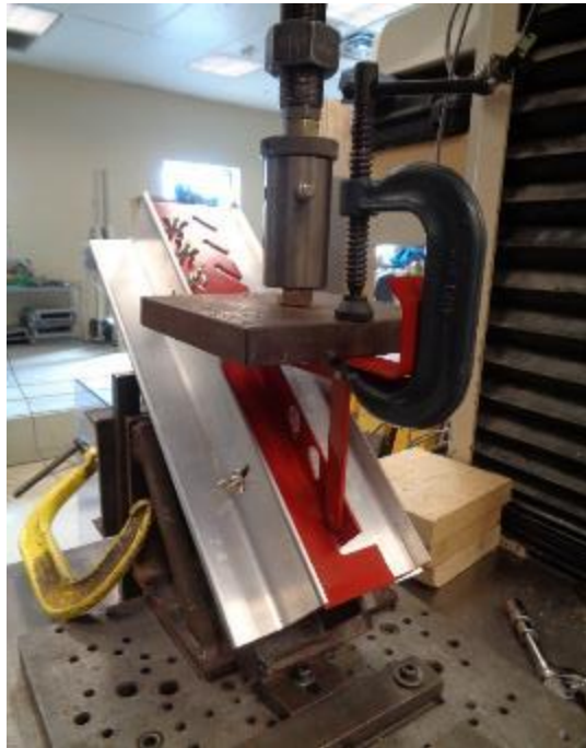
Photo No. 3 Adapter Plate Test - Roof Bracket (with Clamp) - Pre-Test Condition
