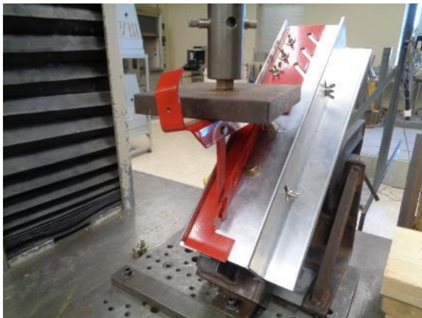
Photo No. 2 Adapter Plate Test - Roof Bracket (No Clamp) - Post Test Condition
