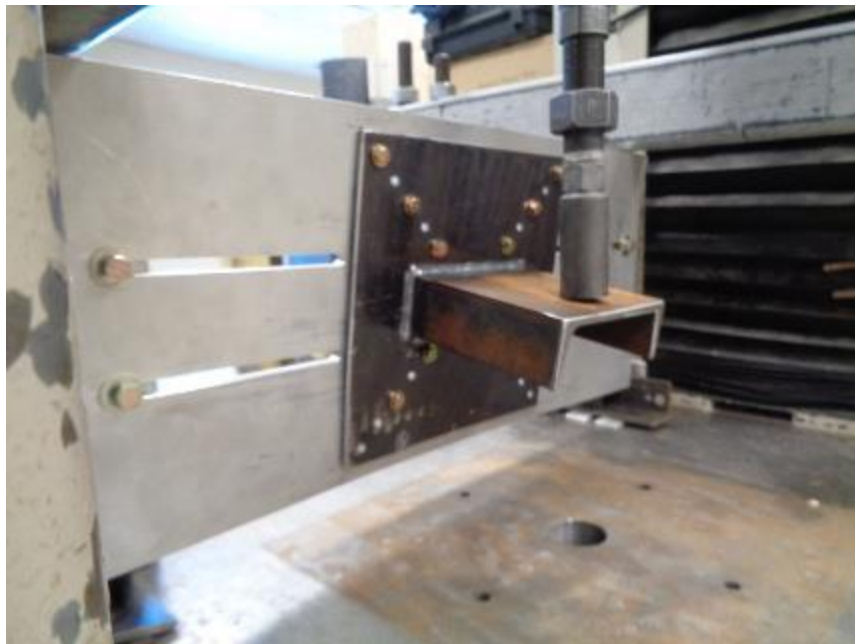
Photo No. 6 Spanner Plate Loading Test in Progress
