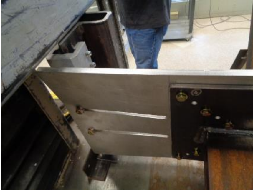
Photo No. 11 Spanner Plate Failure Test in Progress
