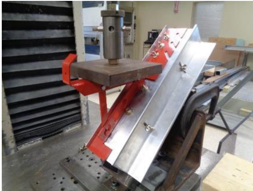
Photo No. 1 Adapter Plate Test - Roof Bracket (No Clamp) - Pre-Test Condition
