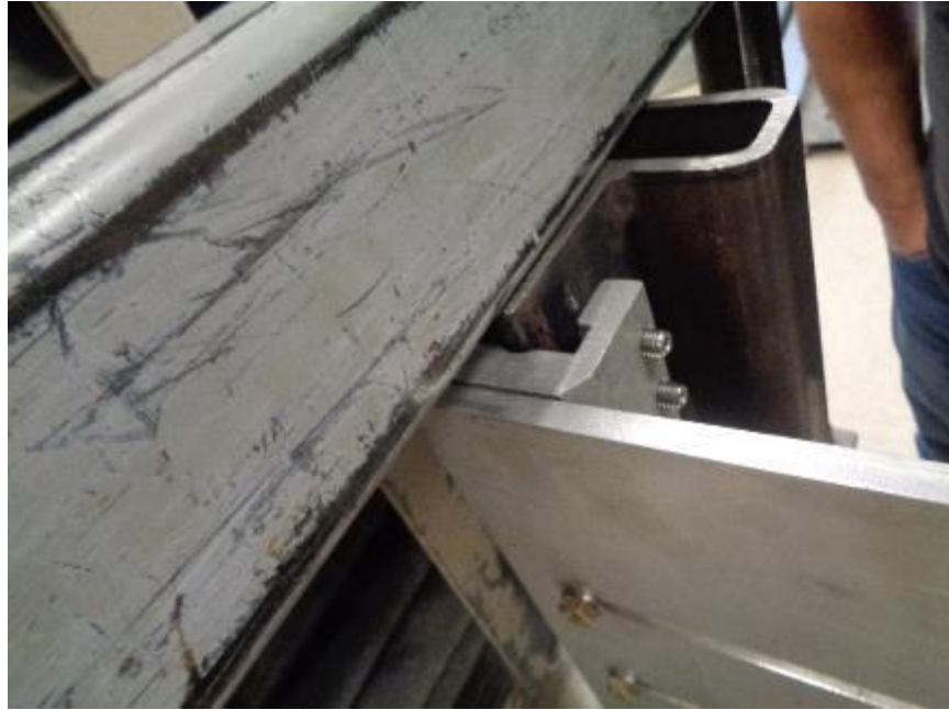
Photo No. 7 Spanner Plate Deflection - 3600 lbf Applied Load
