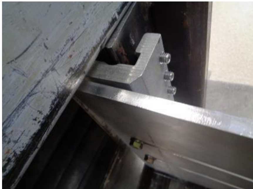
Photo No. 10 Spanner Plate Deflection - 5000 lbf Load Released
