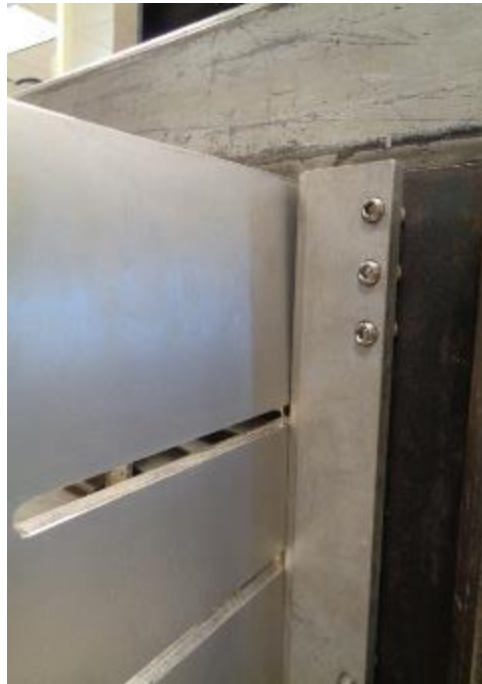
Photo No. 9 Spanner Plate Deflection - 5000 lbf Applied Load
