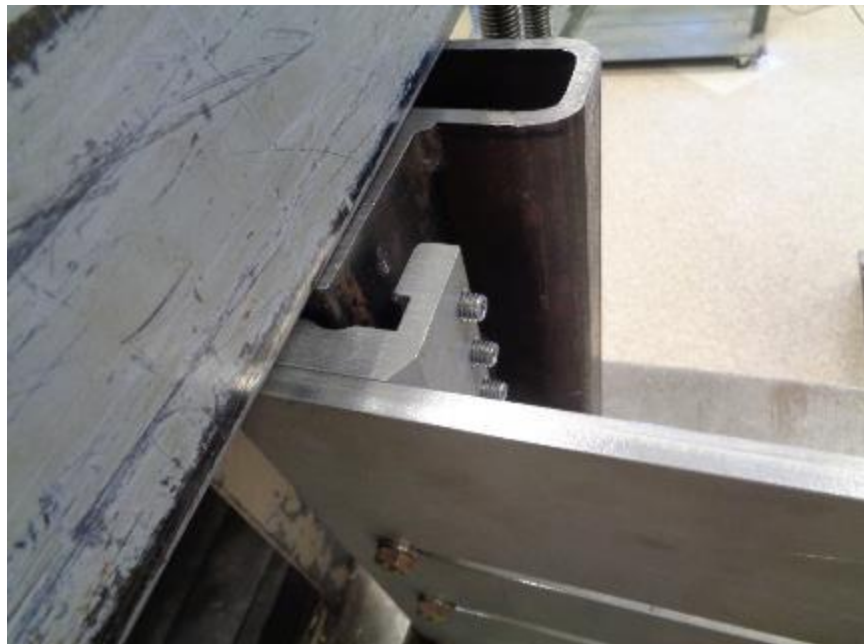
Photo No. 8 Spanner Plate Deflection - 3600 lbf Load Released
