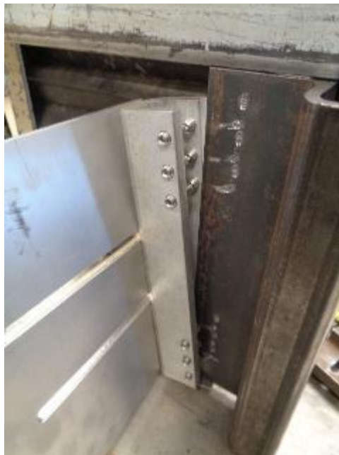
Photo No. 12 Spanner Plate Failure Test - Anchor Failure
