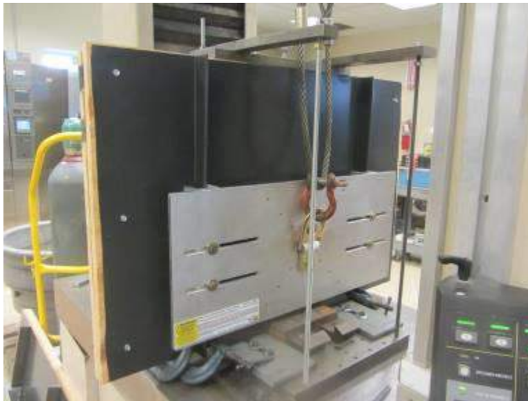
Photo No. 1 Side Load Test Setup - Mockup Anchorage Face
