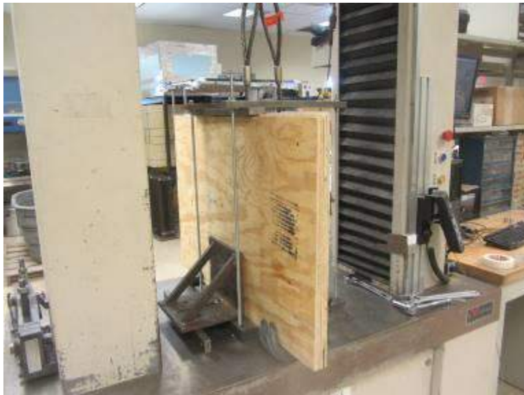
Photo No. 2 Side Load Test Setup - Mockup Rear
