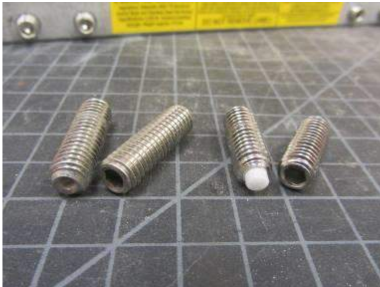
Photo No. 2 Pretest Condition Cupped Tip (Left) and Nylon Tip (Right) Tensions Bolt Details
