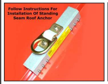
1. Install the Standing Seam Roof Anchors in a straight and level line no more than 8 feet apart. Install according to Standing Seam Roof Anchor instructions and torque to 90 in/lbs for cupped tip set screws and 180 in/lbs for nylon tip set screws. Remove all D-rings, D-ring plates, top bolts, and washers from anchor bodies, if applicable.
