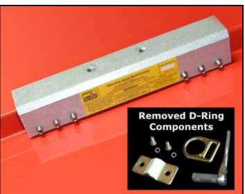
2. Be sure the stabilizer legs on each side of the SSRA2 Adapter Plate are raised to the highest position prior to installation. Using (Grade 8) 9/16-inch top bolts and washers, secure the SSRA2 Adapter Plate to the Standing Seam Roof Anchor body.
