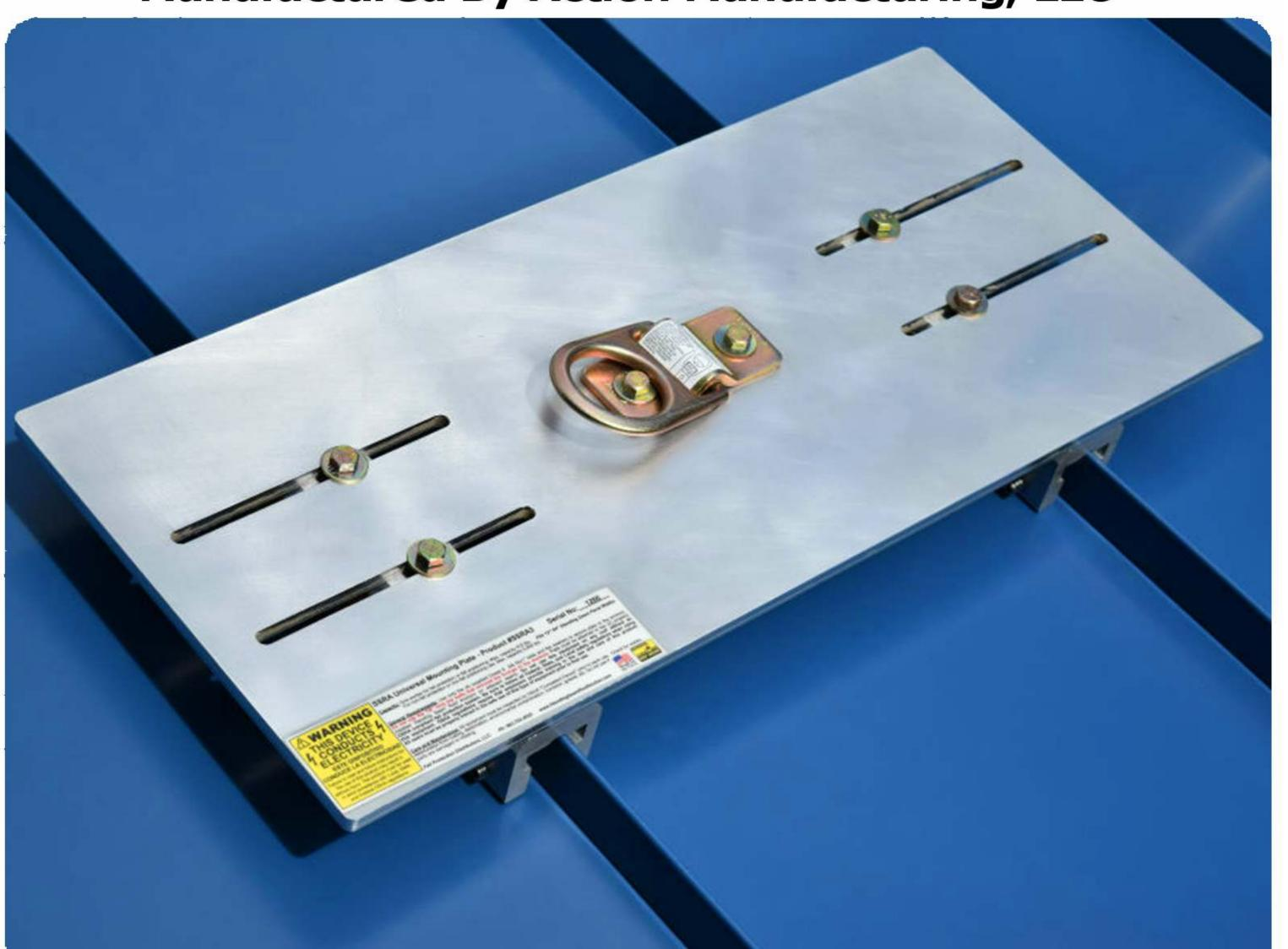
The SSRA3 Anchor Plate is a universal mounting plate constructed of 6061-T6 aluminum and professionally tested to over 10,000 lbs. It can be used to mount anything to a standing seam roof, including fall protection equipment. It is pre-drilled with 4 holes to accept the Falltech 7414 D-Ring (included) mounted either vertically for standard anchoring or mounted horizontally for Horizontal Lifeline attachment.
