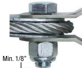
Bolt Thread Penetration
