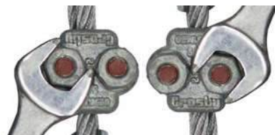
Cable Clamp Tightening
